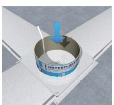
4 | Inserting the shuttering pipe
