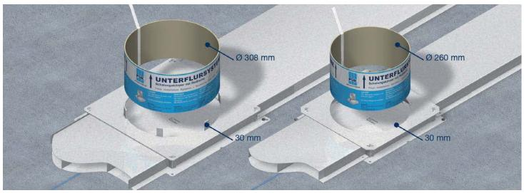
Hollow space floor box for round installation units Ø 305 mm or Ø 258 mm and underfloor ducts of up to 250 or 350 mm width with heights of 28/38/48 mm. Comply with minimum screed covering of 35 mm.
