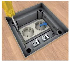
**6 | Heavy current systems** Insert heavy current devices from the top and connect from below. Insert equipped plate using the snap tabs into the frame and fasten the opposite side.
