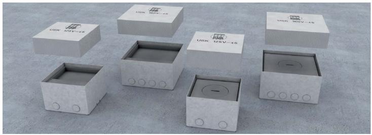
Quadrangular compact single outlet, external dimensions 125 x 125 mm and 160 x 160 mm for installation directly into screed, suitable for dry and wet maintenance rooms. Scope of delivery contains floor box, stainless steel unit and shuttering unit. For parquet and stone floors of 12/22 mm levelling range: 80–125 mm or 90–135 mm.
