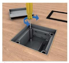
**4** | Levelling to floor Remove cartridge cover and rubber seal and adjust single outlet to floor height flush over the four levelling screws.
