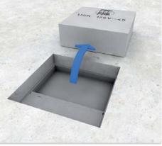
**3 | Casting screed** Seal all openings of the floor box as delivered and cast screed accurately to the shuttering unit. Remove shuttering unit when screed is hardened.
