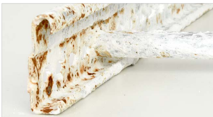
Hot dip galvanized – 1050 h
