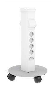
Standard post with four braked castors on a base plate, 4x2-way socket outlets, 5 m connection cord and two empty mounting boxes for data/media.
